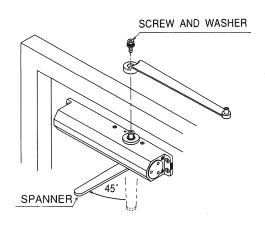
5. SCREW OUT ADJUSTABLE LINK. TURN ADJUSTABLE SCREW CLOCKWISE FOR STRONGER HOLD-OPEN FORCE.TURN ADJUSTABLE SCREW COUNTER-CLOCKWISE FOR WEAKER HOLD-OPEN FORCE.
