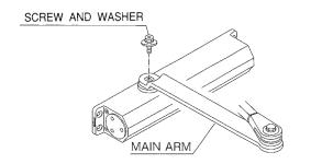
4. OPEN DOOR TO THE DESIRED HOLD-OPEN ANGLE AND FIRMLY FASTEN LOCKING BOLT WITH A SPANNER.
