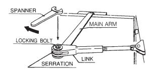
NOTE: DAMAGE TO THE HOLD-OPEN DEVICE MAY OCCUR IF THE LOCKING BOLT IS NOT FIRMLY TIGHTENED.
