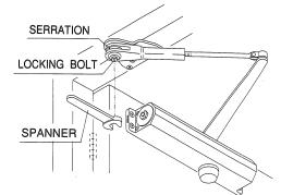
NOTE: DAMAGE TO THE HOLD-OPEN DEVICE MAY OCCUR IF THE LOCKING BOLT IS NOT FIRMLY TIGHTENED.
