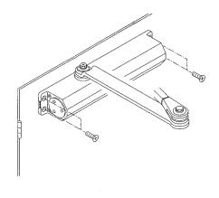
5. SCREW OUT ADJUSTABLE LINK. TURN ADJUSTABLE SCREW CLOCKWISE FOR STRONGER HOLD-OPEN FORCE. TURN ADJUSTABLE SCREW COUNTER-CLOCKWISE FOR WEAKER HOLD-OPEN FORCE.
