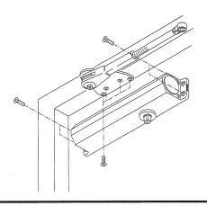
**4.** OPEN DOOR TO THE DESIRED HOLD-OPEN ANGLE AND FIRMLY FASTEN LOCKING BOLT WITH A SPANNER.
