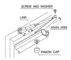
NOTE: ADJUST LENGTH OF ADJUSTABLE LINK TO KEEP CLEAR BETWEEN ARM AND DOOR.
