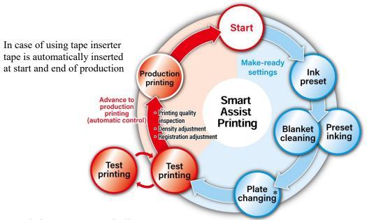
Test printing starts automatically again when the registration and density are out of reference value for production printing.
