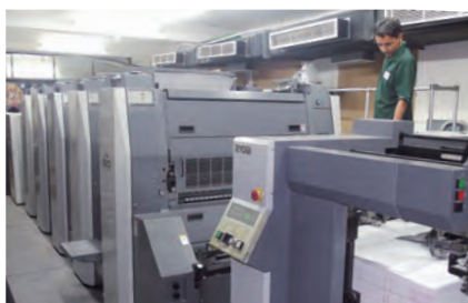
925 A1-size 5-color offset press with LED-UV curing system
