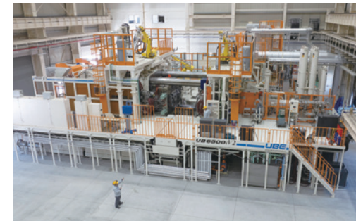
Die casting machine with a clamping force of 6,500 tonnes
