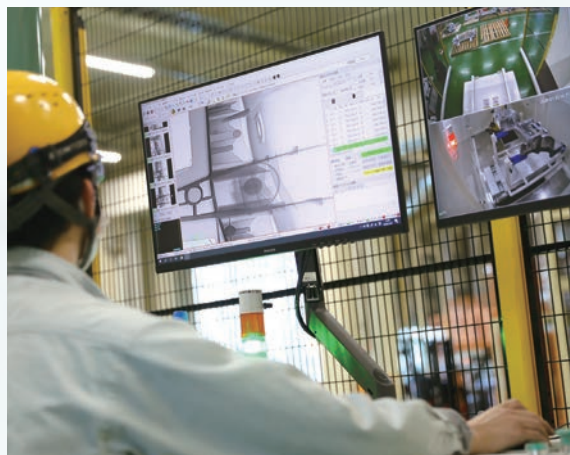
Visualization of internal defects using advanced X-ray inspection system
