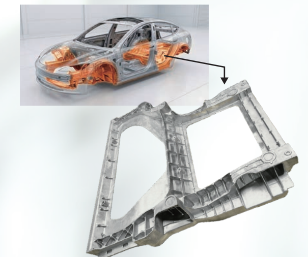
Rear underbody cast using an ultra-large die casting machine. Prototype shown from the underside of the vehicle (148 cm × 134 cm × 37 cm).
