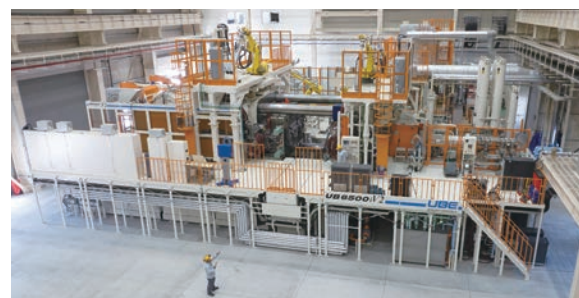
Ultra-large die casting machine with a clamping force of 6,500 tonnes
