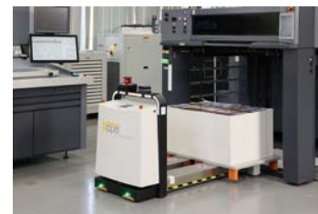
(Left) Coordinating the loading of printing paper and transportation of printed matters with an AGV*
