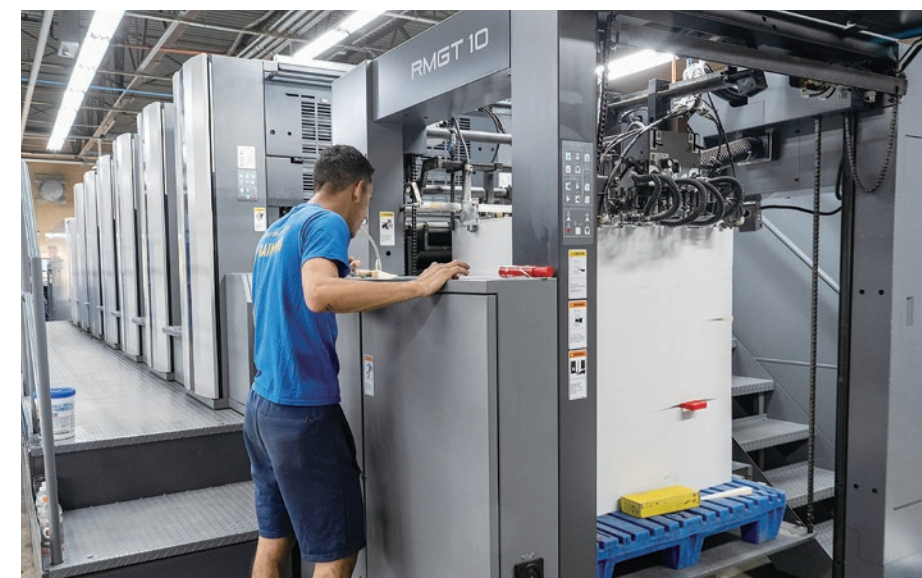
RMGT 1060LX-6 + CC + LD 1,060 mm format wide-stock range 6-color press
