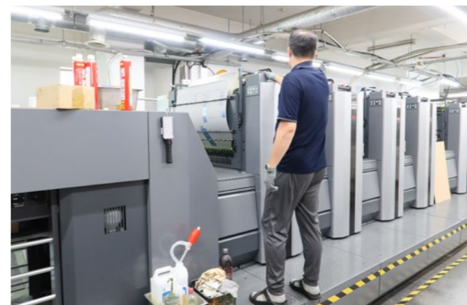
The LED-UV equipped RMGT 970PF-8 has enabled shorter lead times and eco-friendly printing
