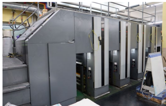
The RMGT 1050TP-8 8-color tandem perfecter has greatly increased productivity for printing fliers
