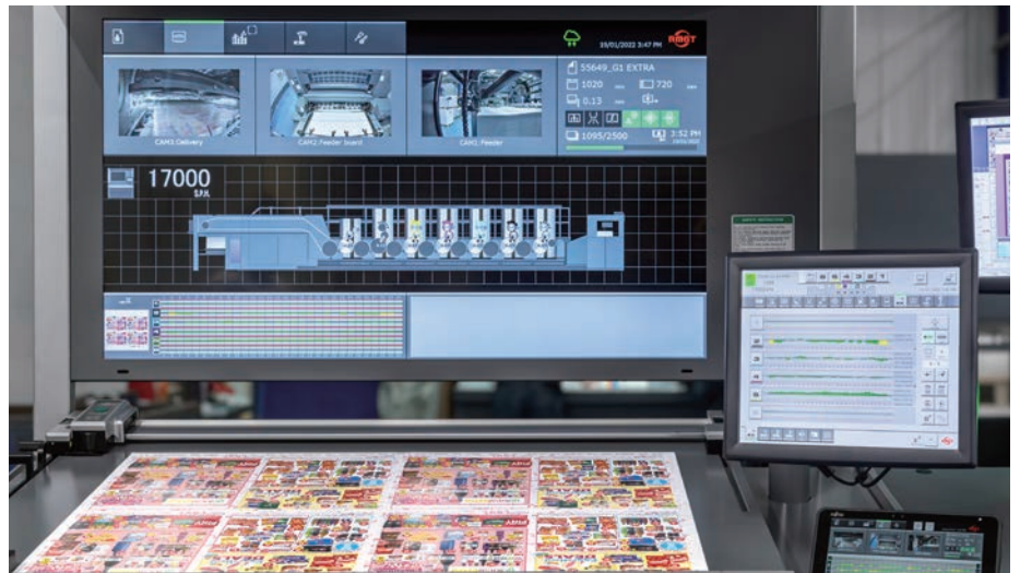
Press Information Display with three network cameras allowing printing status at the delivery
