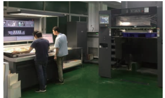
Operators monitoring press operation on a large-screen monitor
