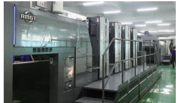
The RMGT 1050AX-4 (front) and 1050AX-5 (rear) presses installed at the new plant
