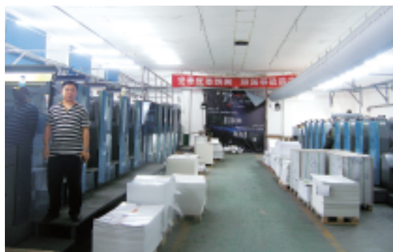
The two new perfectors have greatly enhanced productivity for printing bound materials Left : 1050TP-8 + LED-UV 1050 mm format tandem perfecter Right : 920PF-8 + LED-UV A1-size convertible perfecter
