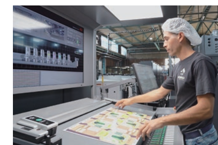
One-pass 7-color printing + varnish coating
